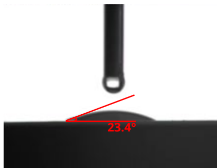
Contact angle of PTFE hydrophilic membrane
