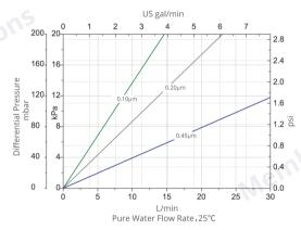
(Water / 1 cP fluid) Typical flow rates. For liquids with viscosity differing from water, multiply the pressure drop by the viscosity in centipoise. Unit conversion: 1 bar = 100 kPa = 14.5 psi
